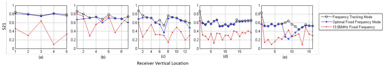
Fig. 3. Comparing optimal fixed frequency mode with frequency tracking and default synchronously tuned frequency modes. a), b) and c) are results for 2-leg-1-hop, 2-leg-2-hop and 2-leg-3-hop, respectively (configurations are shown in Figure 2d-2f). d) and e) are from the sheet relay configuration from Figure 2g and Figure 2h, respectively. The optimal fixed frequency mode is the proposed one in this work.
