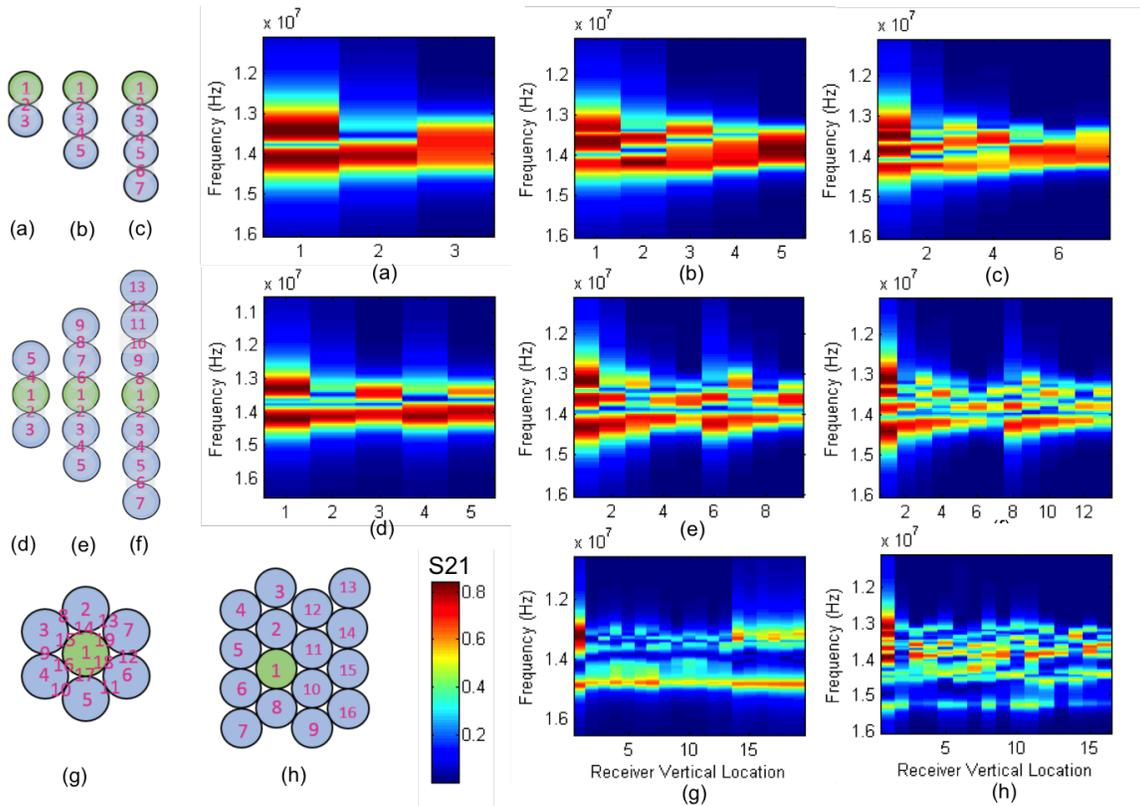
Fig. 2. a), b), and c) are edge-driven 1-hop, 2-hop and 3-hop configurations, respectively. d), e), and f) are middle-driven 1-hop, 2-hop and 3-hop configurations. g) and h) are relay sheet configurations used as points of comparison. S21 response across a frequency range along the relay path is determined for each configuration. In each test, the receiver is located on top of each labeled location in parallel with the transmitter plane, with a separation distance of 37 mm.
