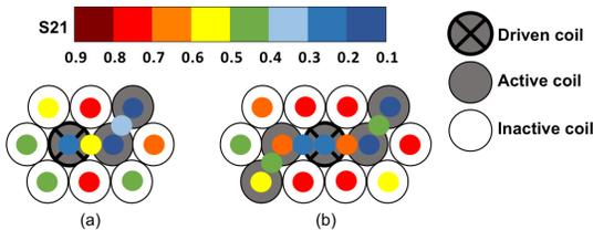
Fig. 5. Compare the S21 at locations that are not directly above the relay path when the receiver has 1cm separation distance from the transmitter plane.
