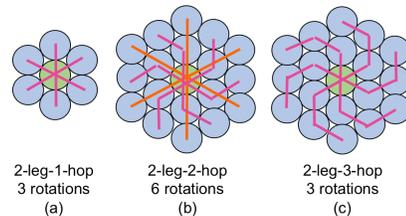
Fig. 6. The proposed time-multiplexing configurations. Each setup uses the middle-driven mode. Through rotation, the entire area is covered. a), b) and c) are 1-hop, 2-hop, and 3-hop, respectively.
