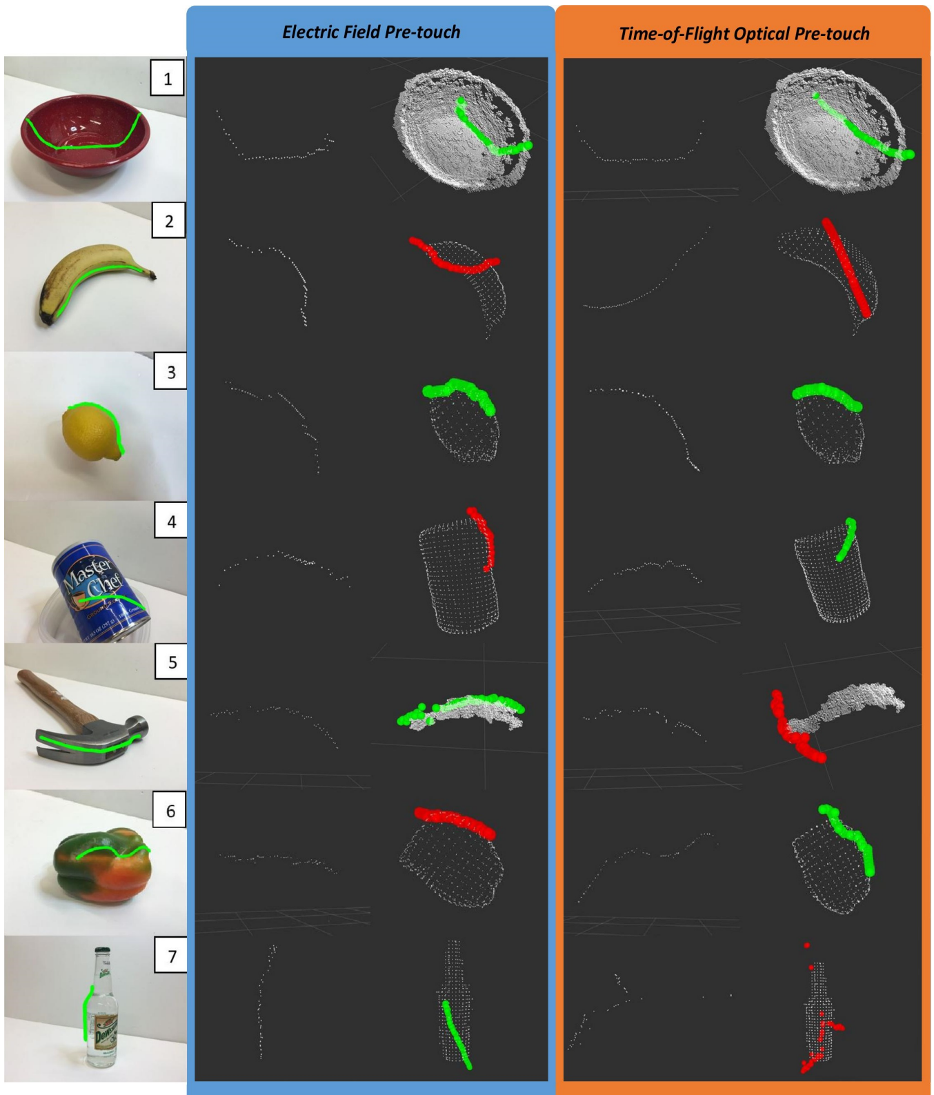
Fig. 5: The results of applying pre-touch scanning and ICP to seven common objects. The first column shows each of the seven objects and the region that was scanned in green. The second column shows the raw point cloud obtained by the electric field sensor for each object, and the third column shows how the ICP algorithm matched the raw point cloud to the reference model. The raw point cloud is colored green if the ICP algorithm found a correct partial or full match, and red if it failed. The fourth and fifth columns display the analogous results for the optical pre-touch scans.
